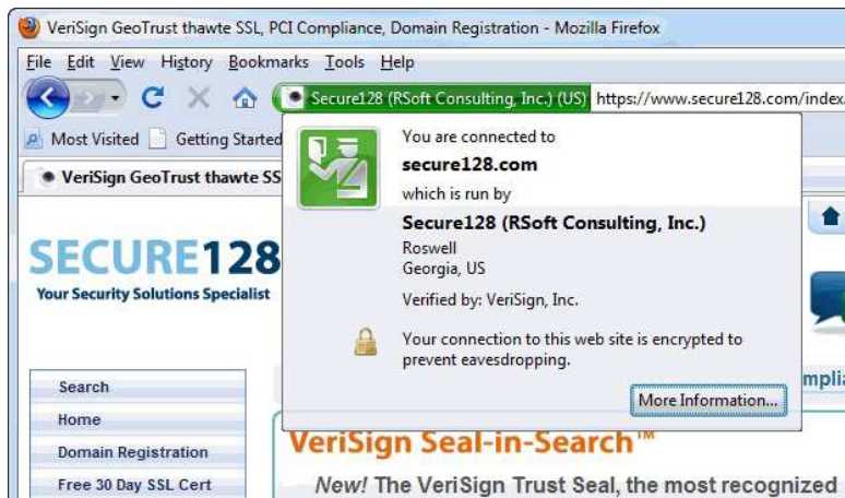
Figure 9.2: When you connect to a webpage protected by SSL/TLS, the Browser displays information on the certificate's authenticity
