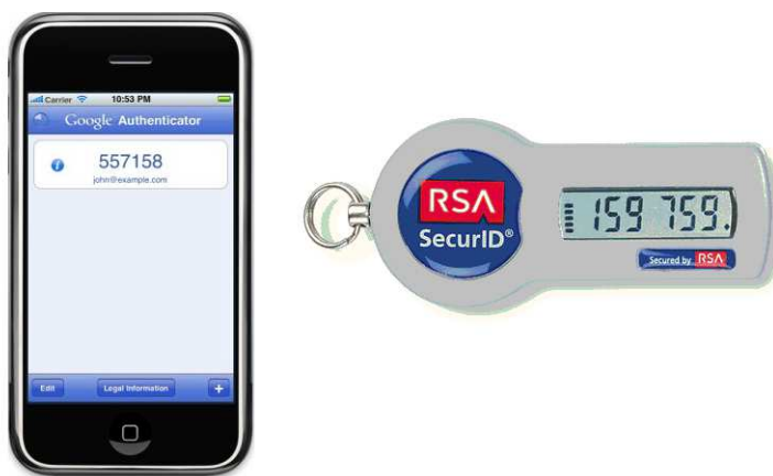
Figure 4.2: The Google Authenticator app is one popular example of a one-time password scheme using pseudorandom functions. Another example is RSA's SecurID token.
